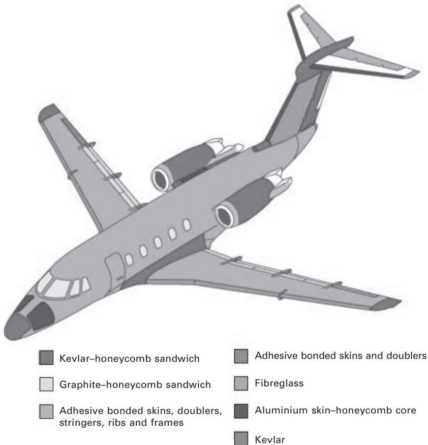
13.13 Application of adhesively bonded sandwich composites in the Citation III aircraft.
