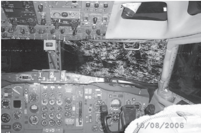
13.10 Hail damage to a cockpit window.
